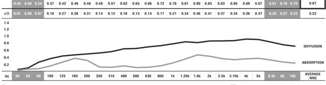
ABSORPTION COEFFICIENT: Values in accordance with the standards: EN 20654, ASTM C423 and EN 11654. DIFFUSION COEFFICIENT: These values were obtained by mathematical calculations and tests carried out in our laboratory
